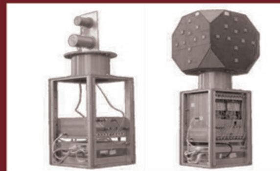
Real-time signal processor of microwave radar for Spacecraft Shenzhou VIII unmanned docking with Space Module Tiangong I
